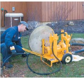
Gorman-Rupp's Tankleenor® provides quick, efficient and economical cleaning of petroleum storage tanks. The unit is a lightweight, wheelmounted cleaning system designed for one-man operation and is easily moved from job to job.
